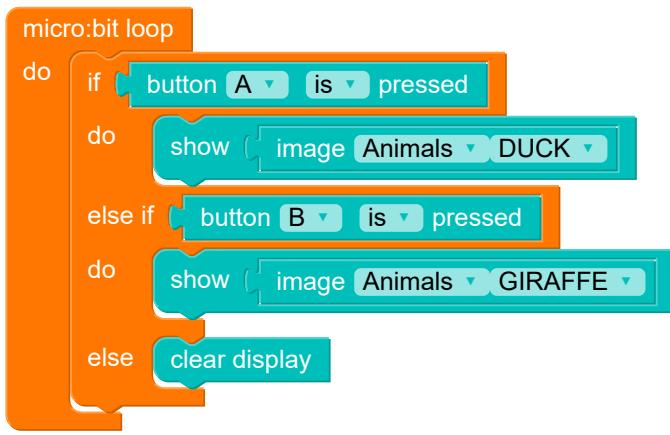
The `if` does button A and shows a duck, and `else if` does button B and shows a giraffe. The final `else` captures all other decisions — in this case, that's just pushing neither of the buttons! Try it out by clicking ► and trying out the two buttons:
