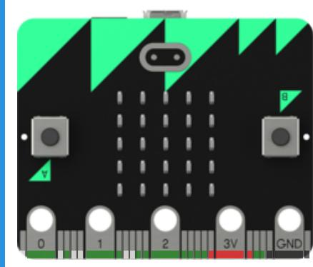
When A is pressed, the image appears. When it is *not* pressed, the image goes away because the program runs `clear display`.
