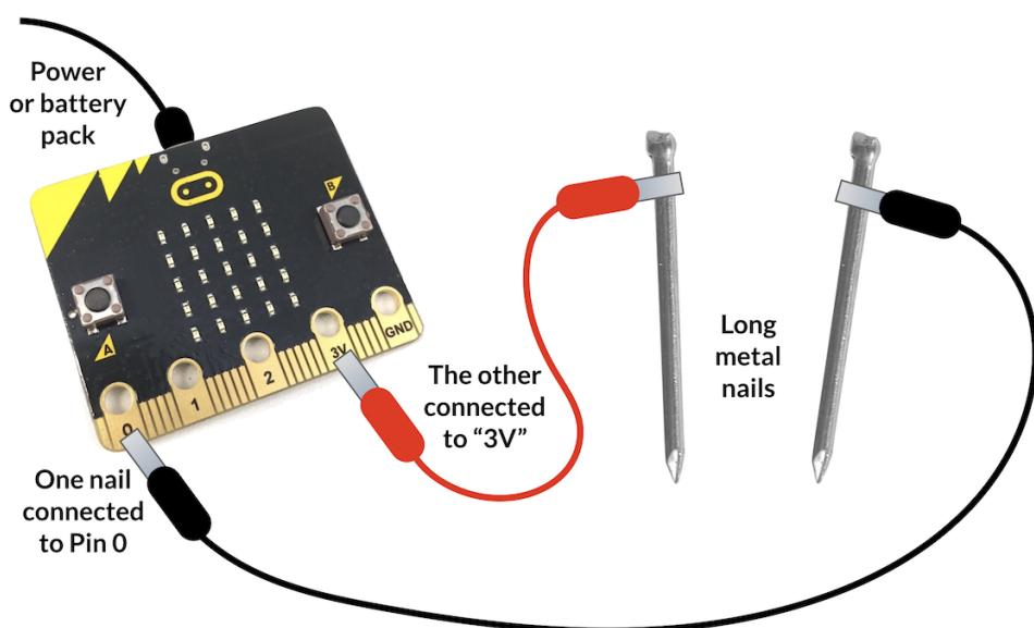
How to hook up the soil moisture probes.
